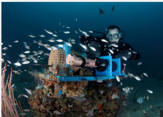
A NOAA Diver works with a seafloor sensor installed in a patch reef. (Photo Credit – Greg McFall)
