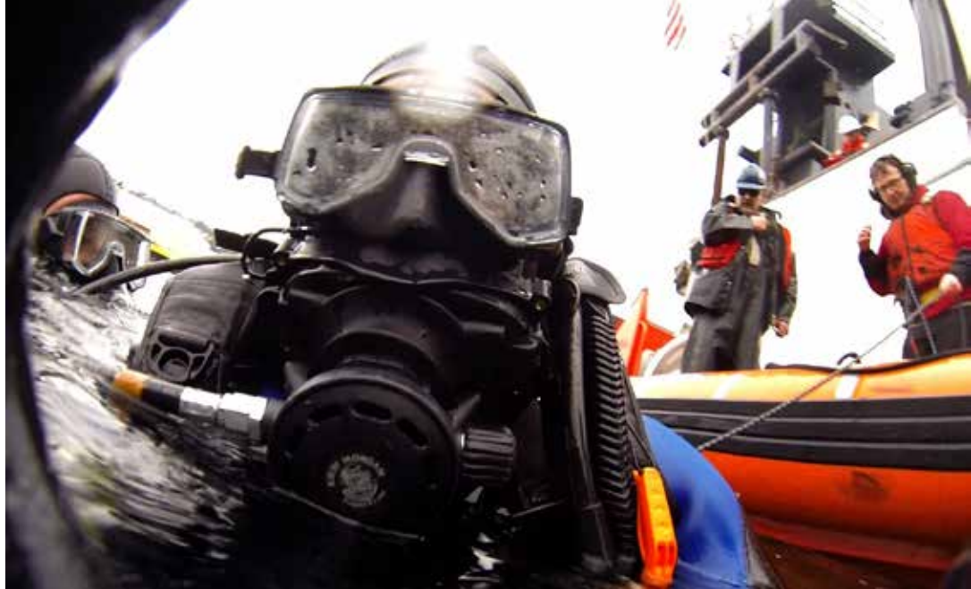
NOAA Corps divers using tethered communications for a hull inspection dive, NOAA Ship Oscar Dyson . ENS Benjamin VanDine, NOAA
