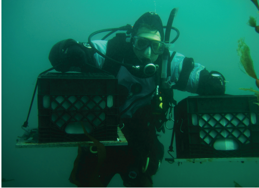
NOAA Diver Chad King retrieving two Autonomous Reef Monitoring Structures (ARMS) from a kelp forest in Monterey Bay NMS. Steve Lonhart/NOAA
