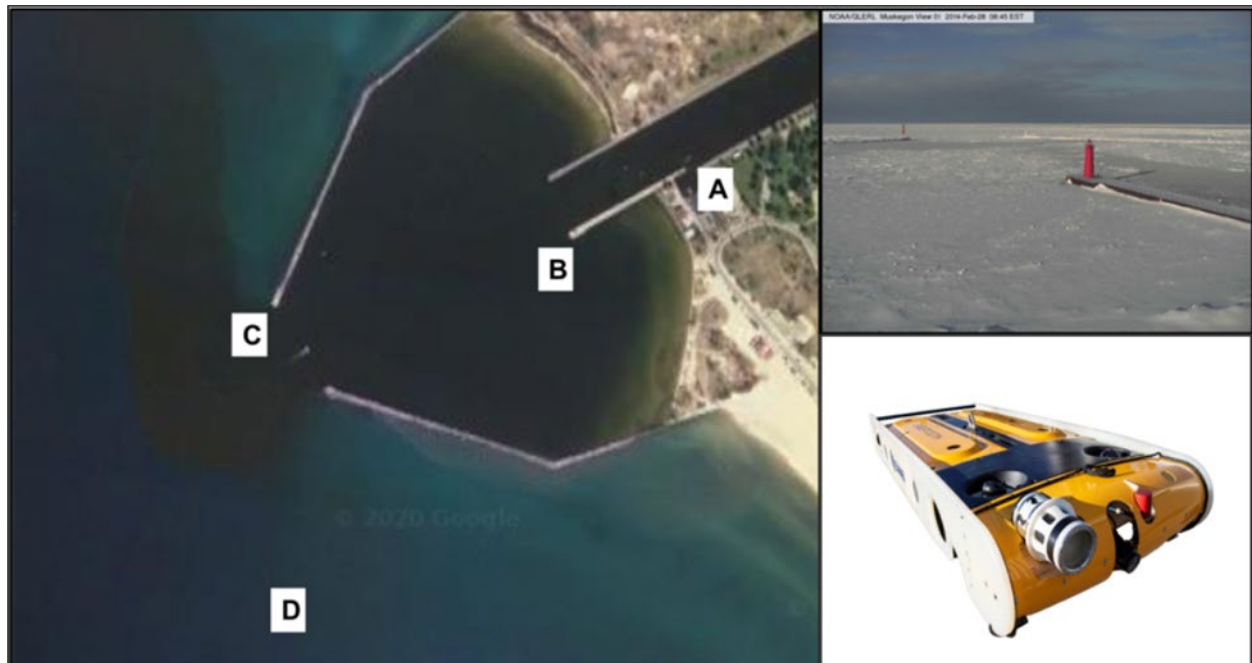
Figure 1: Area of AUV operations including A) GLERL Lake Michigan Field Station, B) future AUV docking station, C) channel entrance, D) mapping area. Image upper right looking A to B; Saab AUV lower right.
