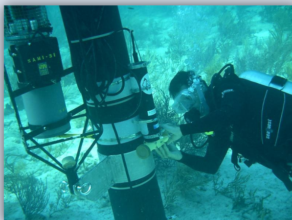
Figure 1: A NOAA Working Diver at the Atlantic Oceanographic and Meteorological Laboratory adjusts a fluorometer at a CREWS station.
