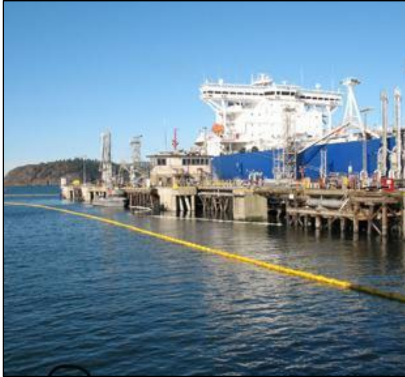
Figure 3.4-3. Booming: deployment of a floating barrier (seen in yellow) to contain marine spills and protect the environment
