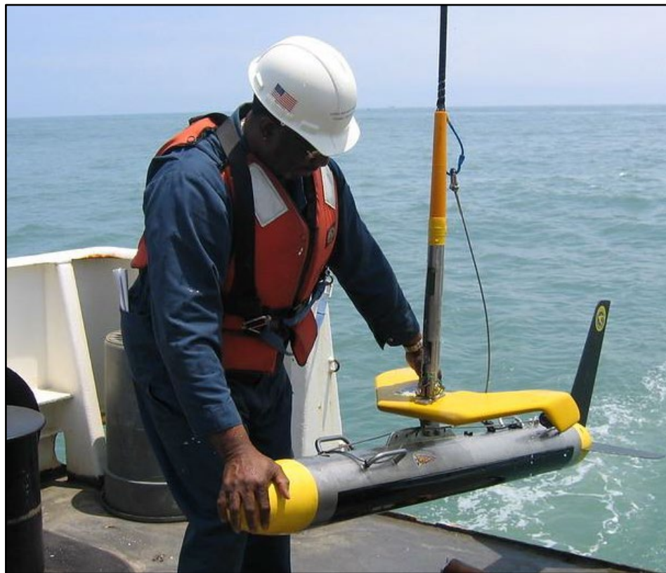
Figure 2.2-1. Side-scan Deployment from NOAA Ship Thomas Jefferson
