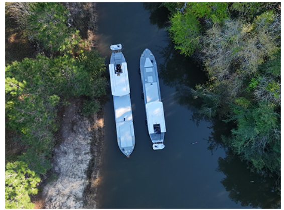
Manned models meeting in a narrow channel to experience bow cushion, bank suction, and squat effects. Photo credit: Grant Begley.
