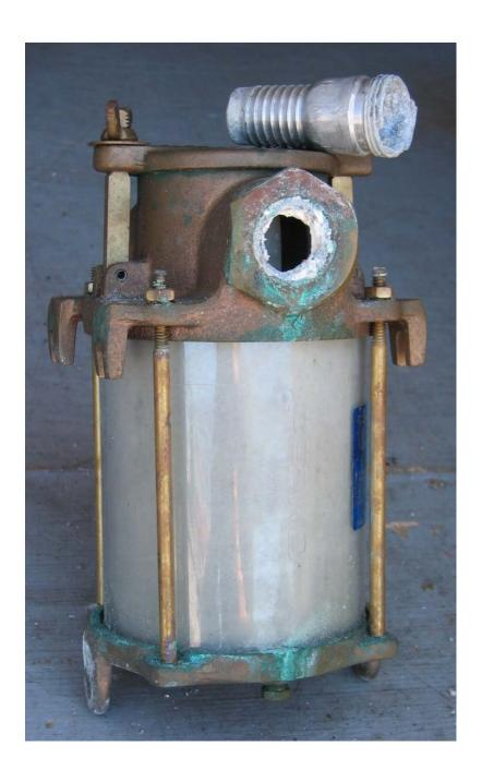
**What is it?** The photo shows the remains of an aluminum hose barb and the bronze sea strainer on which it was installed, in this case in line with the raw water intake hose on NOAA / NRT6s SeaArk Survey Launch S3003, during fabrication.
