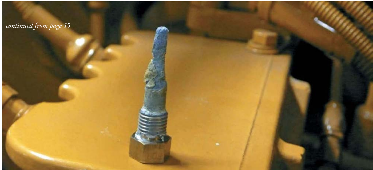
Engine cooling system anodes – These anodes are often hard to locate and therefore neglected. Failure to replace these in a timely fashion can cause serious damage to engine heat exchangers.
