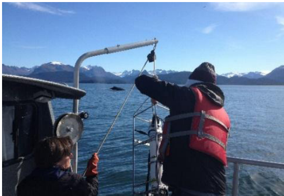
NOAA personnel deploy a CTD—an instrument that measures the water's conductivity, temperature, and depth—in Kachemak Bay, AK, as a humpback whale surfaces. Photo: Domic Hondolero/NOAA
