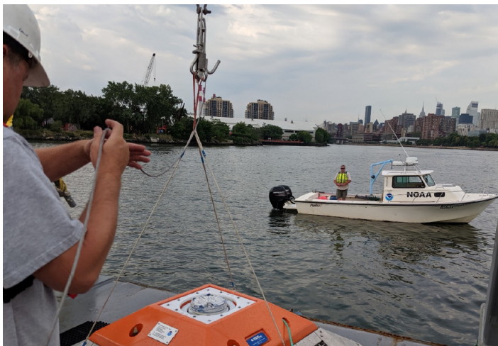
A small boat aids in the deployment of a small portable buoy that collects data for current meter surveys. Photo: NOAA
