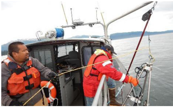
NOAA personnel deploy a drop camera to collect imagery of near-bottom habitats. Photo by Kris Holderied/NOAA.
