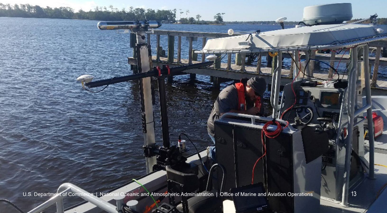
NOAA personnel equip side scan sonar and positioning equipment aboard a small boat. Photo: NOAA
