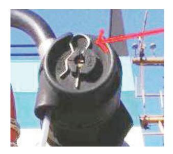
This is an example of a firing head safety pin. Other manufacturers' configurations may differ.
